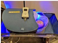
**INMED Photo 1:** The Bili-Kit is a portable, battery-capable toolkit that will allow neonatal jaundice screening, diagnosis and treatment to remote regions that lack access to adequate healthcare.
